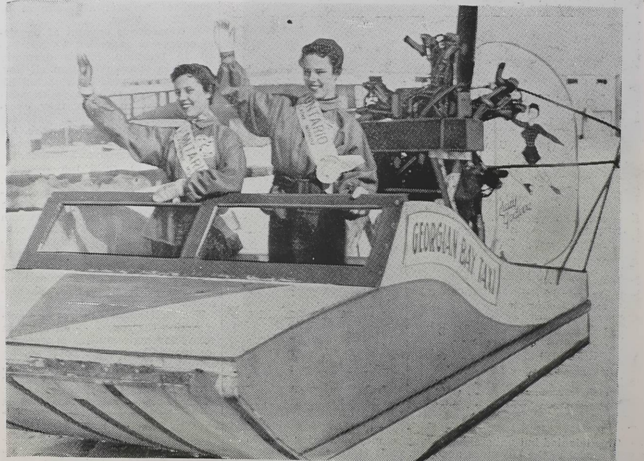
Scoot racing was a feature of the winter carnival of Penetanguishene, Ont., held on March 3. The craft, a sled powered by an airplane motor in the rear, reaches speeds of 120 mph on ice and snow and they gave spectators a thrill as they bounced and turned on the race course.
